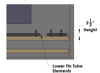
c.) Hang the upper Fin Tube Elements by placing it gently onto the Fin Tube Mounting Brackets. The tubes of the Fin Tube Elements will rest in the V-Groove of the Fin Tube Mounting Brackets. The Fin Tube Elements are 2.75" fin width and 2.50" fin height. Make sure the Fin Tube Elements are positioned in the correct orientation.
