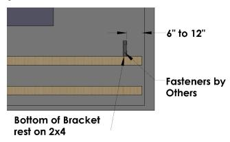
b.) Hang the lower **Fin Tube Elements** by placing it gently onto the **Fin Tube Mounting Brackets**. The tubes of the **Fin Tube Elements** will rest in the V-Groove of the **Fin Tube Mounting Brackets**. The **Fin Tube Elements** are 2.75" fin width and 2.50" fin height. Make sure **the Fin Tube Elements** are positioned in the correct orientation.
