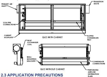
When in cooling mode, the entering water temperature to the QLCI displacement induction ventilation diffuser coil should be maintained warmer than the space dew point temperature in order to prevent condensation.
