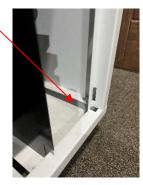
d.) If inspection of the Fin Tube Elements is needed, remove the Rear Fin Tube Element Grill on the back of the QLCI. Locate the (2) socket head screws on the top of each Rear Fin Tube Element Grill. Loosen the locking screws using an 5/32" Allen Wrench and remove the QLCI Rear Fin Tube Element Grill as shown below. Make sure when placing the QLCI Rear Fin Tube Element Grill back in place that the side tabs interlock with the metal flanges.
