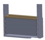
A custom front panel designed for a fan coil renovation project with strict dimensional tolerances between wall cavities in a high demanding dorm room environments.
